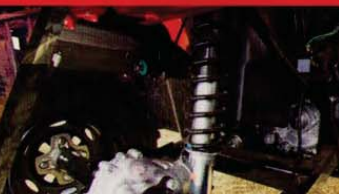
Longer suspension travel for increased ground clearance
